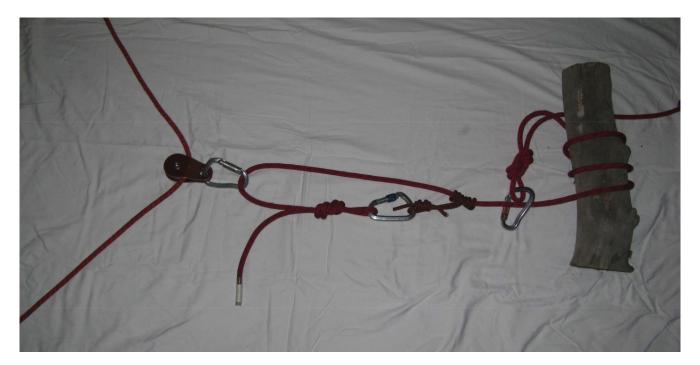
Adjustable change of direction. Moving the prusik on the fixed anchor moves the pulley closer to or farther from the anchor.
