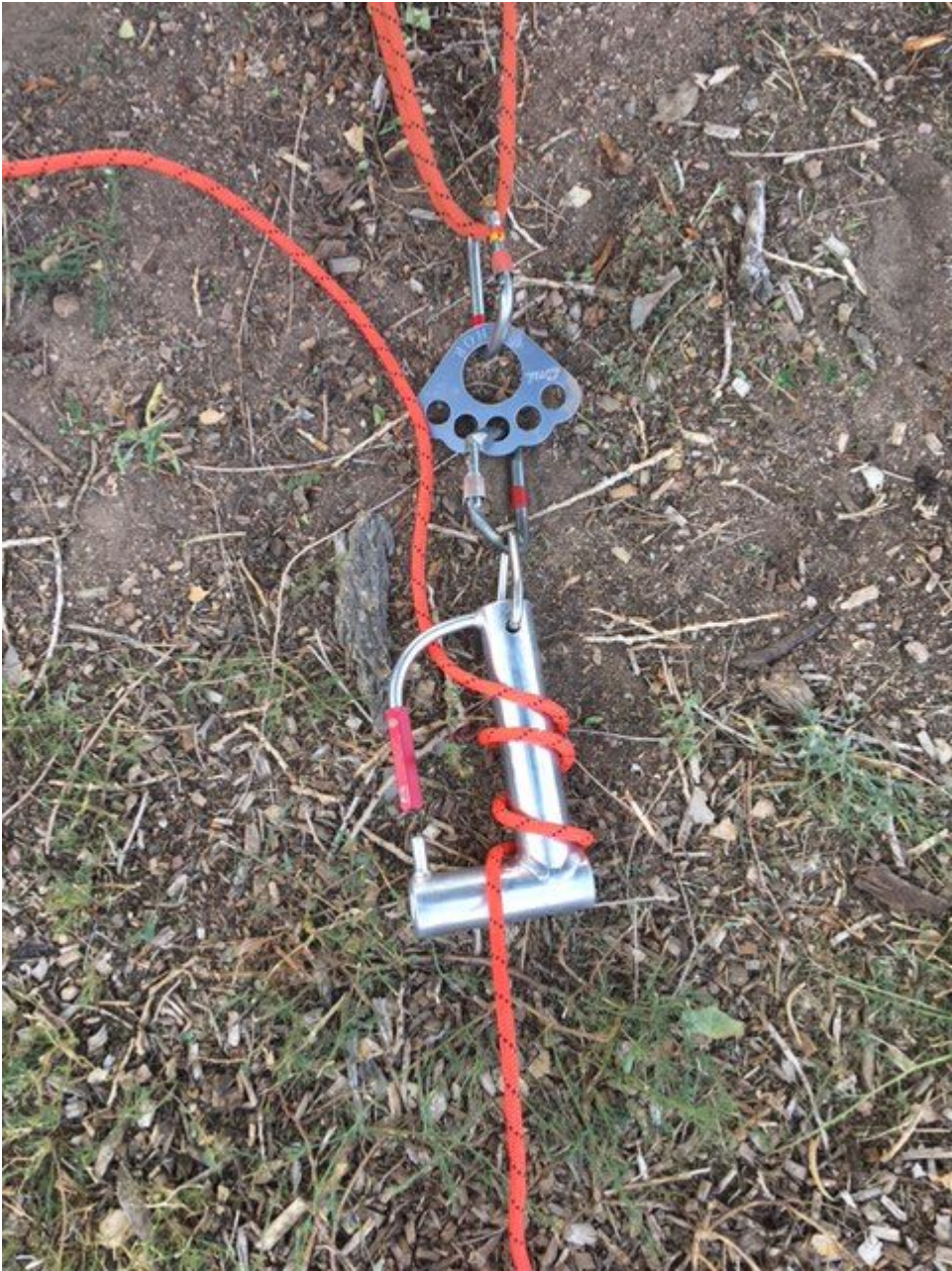
■ Rigging plate with brake for lowering system
