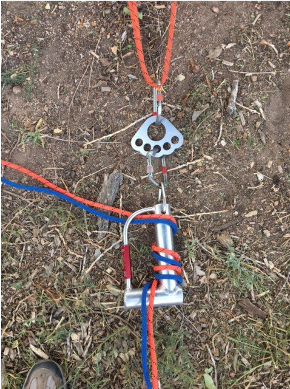
Two ropes wrapped on Brake Tube.
