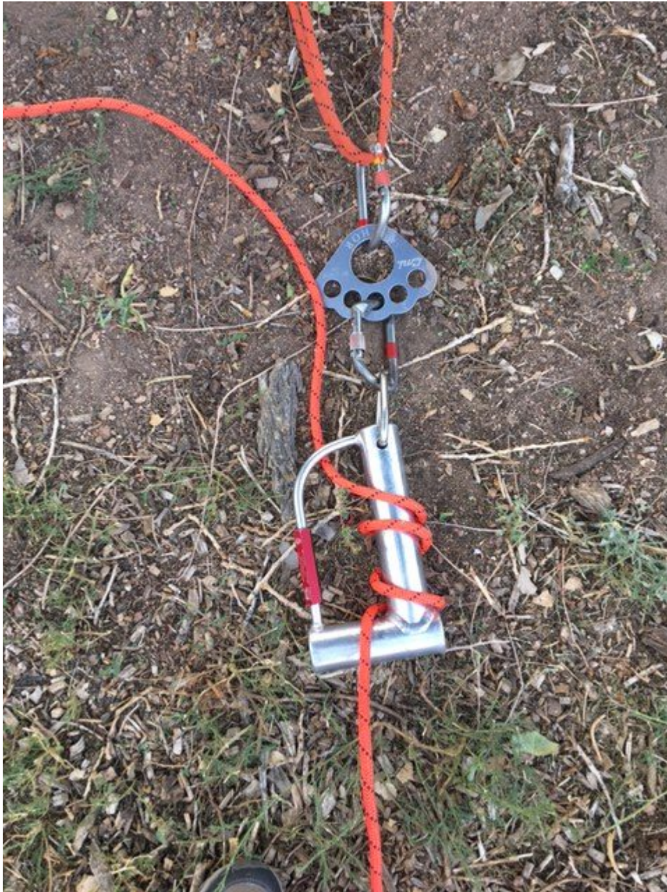
Single rope wrapped on Brake Tube. Red sleeve closed during operation
