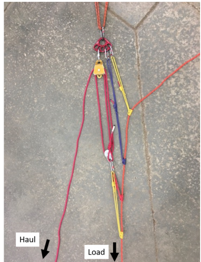
Piggyback uphaul system with 3 to 1 mechanical advantage. (a.k.a. "Z" rig) Left system without Change of Direction. Right system with Change of Direction
